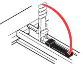
IMPORTANT: Before folding the second section of the tonno, rear clamps must be stowed into the rear bow to prevent damage to fabric.
